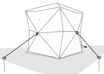
The unique hexagonal head of the Falcon Pins allow for easy tie down of guy wires for securing ground blinds, tents, or other lightweight structures. Install with a hand drill. The unique coil shape is designed for optimum pull-out strength in varying soil types.
