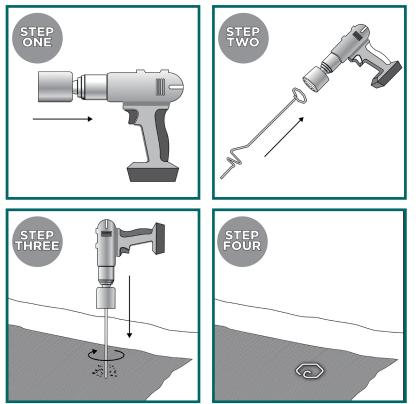
The Falcon Hex Pins are an innovative fastener providing significantly greater pullout resistance than typical straight pins or staples. Falcon Hex pins install using a cordless hand drill with our custom installation chuck or a standard 1.5" hex socket (pictured).
